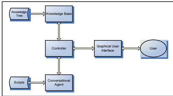
Figure 1: CES system structure.
